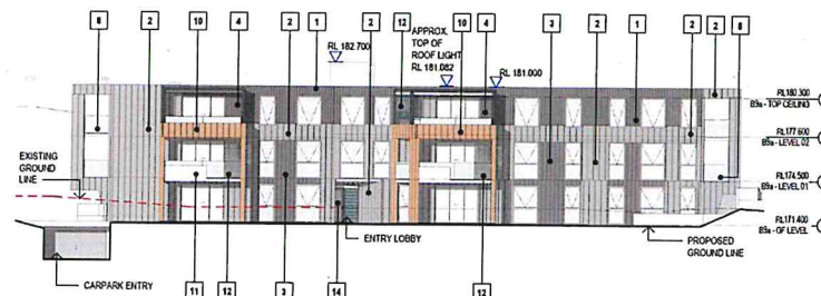
3 BUILDING 9A - EAST ELEVATION 1
